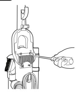
Screw handle in place with the screws provided.
