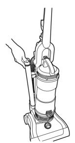
Attach the extension tube/crevice tool to cleaner.
