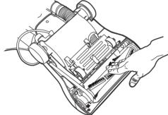
Remove brush assembly and check for wear on the belt. Loop the new belt around the motor and brush channel.
