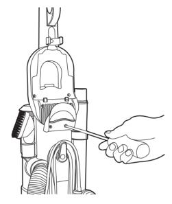
Attach and screw hose hook in place.
