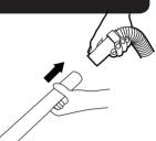
Check the hose by removing it from the cleaner, stretching it to full length.
