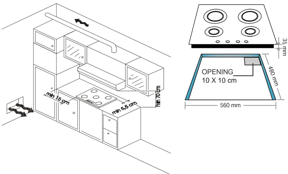
The body of the hob is fitted with 4 location holes to take the fixing brackets that secure the hob in the unit. Place the 4 fixing brackets in such a way that the hob is placed perfectly in the support unit.
