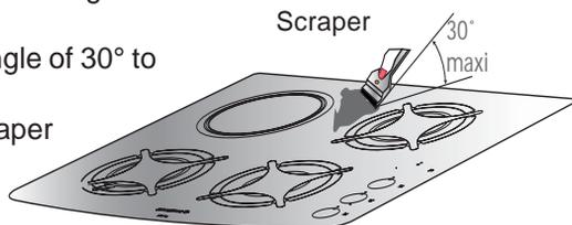
A scraper with a razor blade will not damage the surface, as long as it is kept at an angle of 30°. Never leave a scraper with a razor blade within the reach of children.
