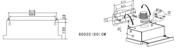
4. Fix the one-way-valve to the air outlet of the cooker hood.
