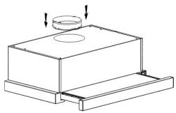
2. Mount the cooker hood on the cabinet by 6 screws (4x35mm) and flat washers.
