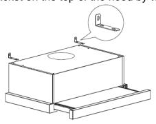
3. The cooker hood is wall mounted by 4 screws (4mm x 30mm) and wall plugs. Mount the cooker hood on the wall on the back of the cooker hood by 2 screws (4mm x 30mm) and wall plugs. Then fix the cooker hood on the wall by 2 screws (4mm x 30mm) and wall plugs through the small L-shaped bracket.
