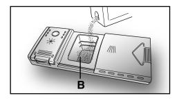
After pouring the detergent into the container, close the lid, firstly pushing (1) and then pressing on it (2) until you hear the click.
