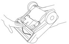
Refit the brush guard with 6 retaining screws.
