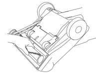
Rotate the brush to ensure free movement of the belt.
