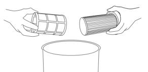
3 Remove the protective filter mesh from the HEPA filter, then gently tap both filters to release any excess dust.
