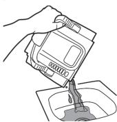
WARNING: Always switch the cleaner off and unplug it from the electrical sock before emptying the dirty water tank.
