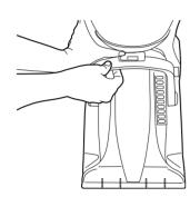
Turn the tank cap anti-clockwise to open.
