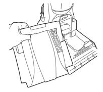
Empty the tank. Rinse the tank with clean water and allow to dry before storing the cleaner.
