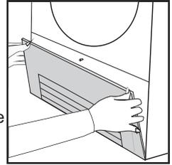
2. Turn the two locking levers anti-clockwise and pull out the front cover.
