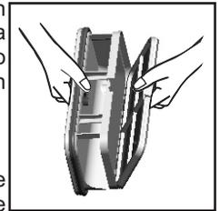
4. Remove the sponge gently from its place and then wash the sponge by holding it under a running tap turning it so to remove any dust or fluff.
