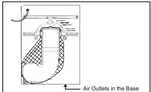
**Important:** During transport ensure that the dryer is in an upright position, if it's necessary you can only flip in the side shown;
