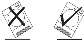
**Caution:** If the product is in different side, wait at least 4 hours before switching on so that the oil can flow back into the compressor. Failure to do this could result in damage to the compressor.
