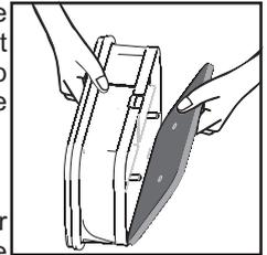
5. Refit the front cover ensuring it is in the correct way (as indicated by the arrow) and pushed firmly into place. Lock the two levers by turning them clockwise.
