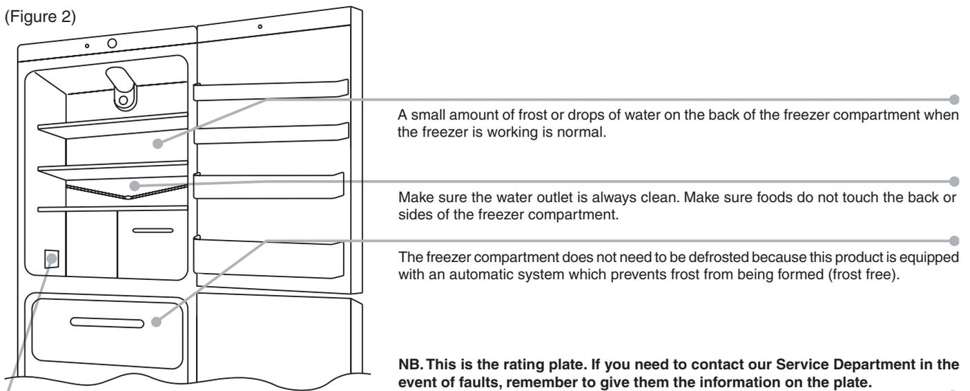
A small amount of frost or drops of water on the back of the freezer compartment when the freezer is working is normal.
