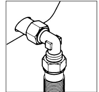
3) Attach fitting C to mains gas supply using rigid copper pipe or flexible steel pipe.
