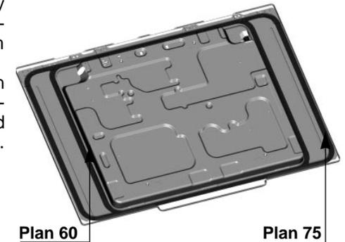
**Important - The diagram below shows how the sealant should be applied.**
