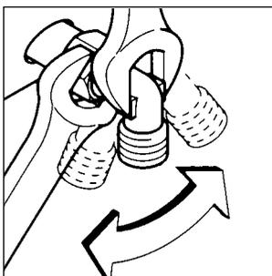
2) Tighten the joints with the Spanners, remembering to twist the pipes into position.
