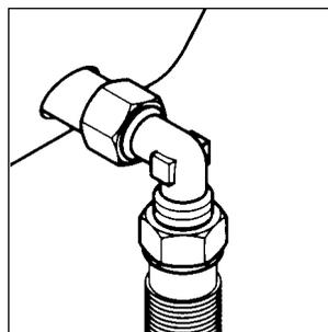
3) Attach fitting C to mains gas supply using rigid copper pipe or flexible steel pipe.
