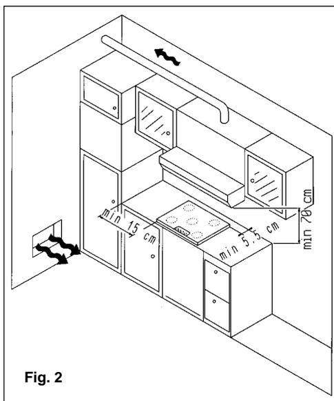
If a hob of 60 cm is fitted above an oven which is not equipped with fan cooling system it is recommended that openings are created within the built in furniture to ensure correct air circulation.
