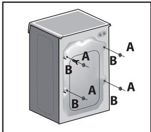
**Step 3.** Remove the 4 retaining screws at the rear of the machine, as indicated in the image on the left. Use the blanking plugs provided in the instruction booklet pack to cover the holes once the screws have been removed.
