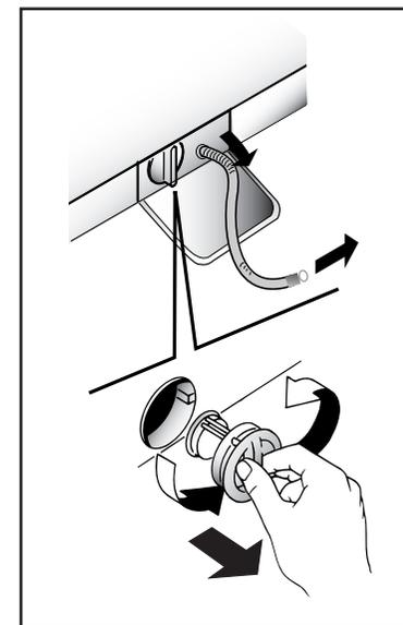
**Step 4.** Turn the filter anti-clockwise until it stops in the vertical position. Remove the filter and clean.
