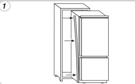
Install the appliance in the unit, Aligning it on the opposite side from the hinges.
