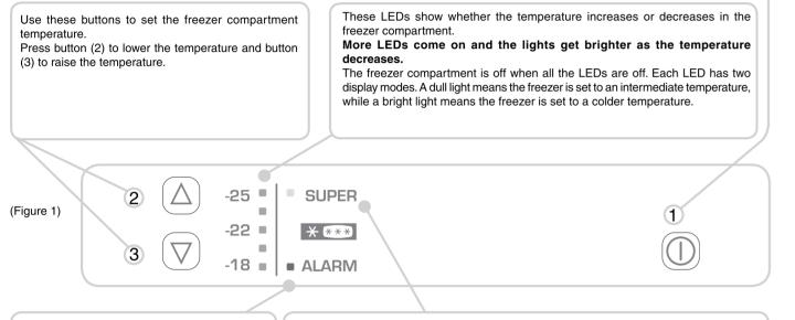
The red alarm light comes on if the freezer compartment temperature is -7°C. If the temperature goes below -8°C the fight will automatically turn off.
