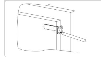
Fit the appliance door to the door of the unit, using the slots on the slide bracket as a guide.
