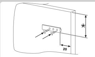
Open the doors of the unit and fridge. Position the slide bracket around the slide and secure to the appliance door.
