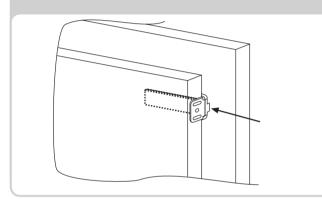
Mark the holes for the screws and drill with a 2.5 mm diameter bit.
