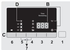
**A-Programme Selector -** Rotating the knob in both directions it's possible to select the desired drying program. To cancel the selections or switch off the dryer rotate the knob on OFF.
