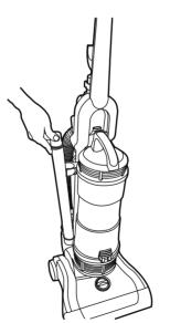
Attach the extension tube/crevice tool to cleaner.
