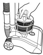
Remove the dust container rotate and remove the exhaust filter cover.
