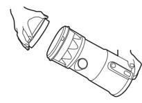
Remove the filter assembly from the dust bin.
