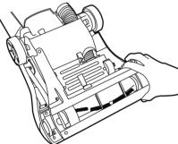
Rotate the brush to ensure movement of the belt.
