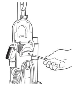
Attach and screw hose hook in place.
