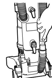
Removing a blockage from the pet hair & allergen remover. Open the nozzle at each side, lift cover and remove the blockage.
