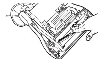
Check for a blockage in the hose socket. Use a flexible rod to remove any obstruction.
