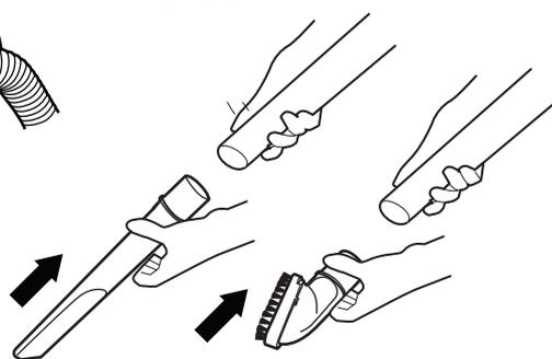
6 Fit the pet hair & allergen remover\* Fit the hard floor caresse nozzle\* to the crevice tool.
