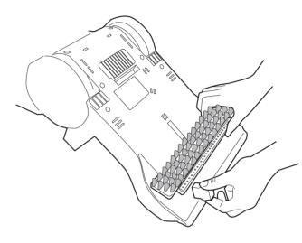
Replace the brush bar and attach to the nozzle. Attach the alignment brackets and assemble to the cleaner.
