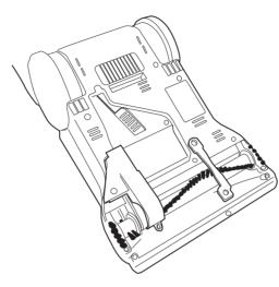
Replace the agitator by looping the belt around the agitator making sure it sits securely in the belt channel.
