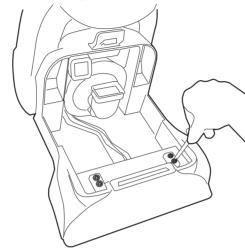
Unscrew 2 retaining screws located on the underside of the detergent nozzle. Remove the brushbar from the nozzle.
