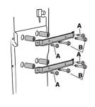
Remove the 4 screws (A) from both clamps and the 4 screws (B).
