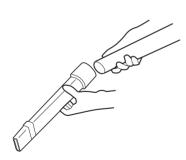
Attach crevice tool to the end of the telescopic tube\*.
