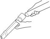
Check the hose by removing it from the cleaner, stretching it to full length.
