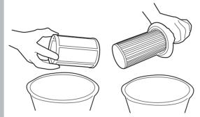
Gently tap both filters to release any excess dust.
