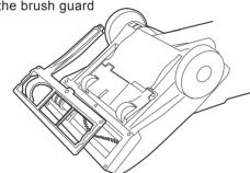
Rotate the brush to ensure movement of the belt.
