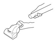
**IMPORTANT!** When using cleaning tools, the cleaner must be kept in the upright position, particularly when cleaning stairs. The nozzle height should also be set to tool mode.
