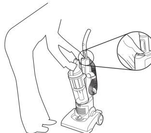
Hold the container over the bin and press the bin open button .
