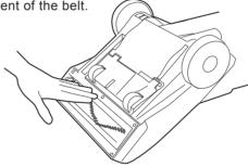
Remove brush assembly and check for wear on the belt.
