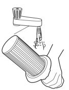
Wash both filters under hand warm water until the water runs clean. Remove excess water by shaking and leave to dry for 24 hours.
