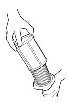
Remove the mesh filter from the filter assembly.
