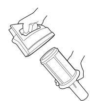
Remove the filter assembly from the upper part.
