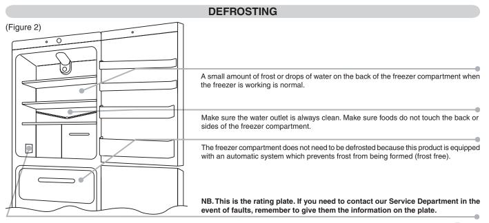
Important: If the room temperature is very warm, the appliance may work continuously and a layer of frost will deposit on the back of the fridge compartment. In this case, turn the knob to lower settings (1-2).
