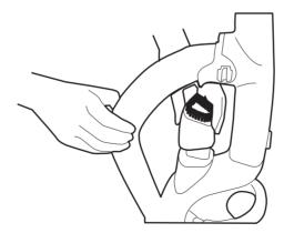
Connect the handle to the top of the machine by pressing down firmly until it clicks into place.
