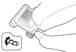
The brushbar rotation automatically stops when the cleaner is put into the upright position.
