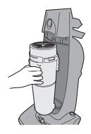
Remove the dust cassette from the cleaner using the handle grip on the front.
