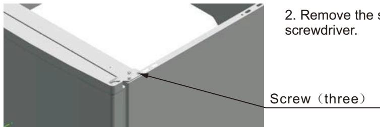
2. Remove the screws fixed the top-hinge with cross-slot screwdriver.
