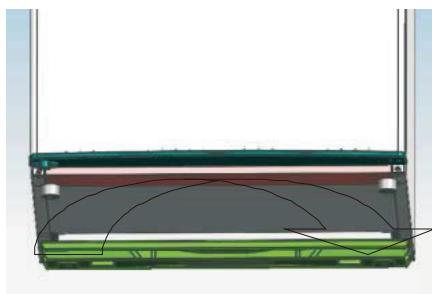
12、replace the leveler to the other side and adjust it to make sure the cabinet level
