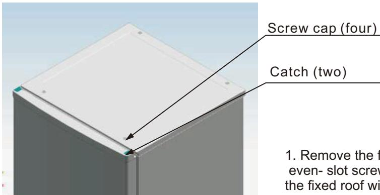
1. Remove the four screw caps and two catches with the even-slot screwdriver. Then disassemble the screws top the fixed roof with the cross-slot screwdriver.
