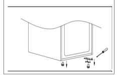
4. Remove the right door stopper on the bottom of fridge and freezer door, then get the left door stopper from the accessory bag, install it on the bottom left side of fridge door and freezer door. Remove the pin shaft and install to other side.
