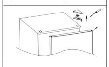
2. Remove two screws that secure the center hinge.
