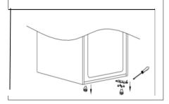
4. Remove the right door stopper on the bottom of fridge and freezer door, then get the left door stopper from the accessory bag, install it on the bottom left side of fridge door and freezer door. Remove the pin shaft and install to other side.
