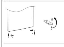
5. Remove the freezer right hinge hole cover, install to lest side. Remove the center hinge screw hole plug on the left side, then install its to right side,
