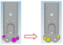
This situation apply to open door in right side This situation apply to left side **Assemble the refrigerator door and freezer door to the opposite side**
