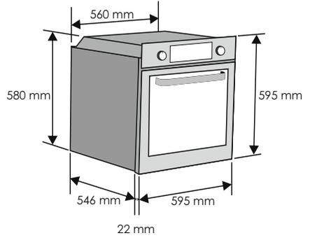
**A EN** If the mounting of the plinth does not allow air circulation, to obtain the maximum performance of the oven it is necessary to create an opening of 500x10mm or the same surface in 5.000mm<sup>2</sup>
