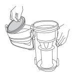
3 Gently tap both filters to release any excess dust.
