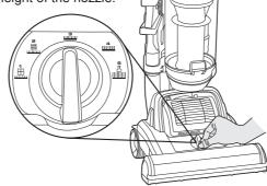
Ensure that the cleaner is in the upright (parked) position and move the selector to the required setting for the carpet type or floor covering.
