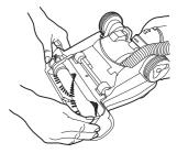
Rotate the brush to ensure free movement of the belt.
