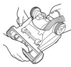
Remove brush assembly and check for wear on the belt.
