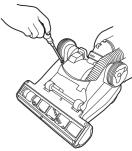
**NOTE:** If the brush is blocked and has stopped rotating, switch off and remove the plug from the electricity supply, then use a pair of scissors to cut through any threads or hairs caught around the brush. Reassemble the brush and brush guard.
