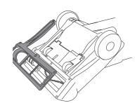
Remove brush assembly and check for wear on the belt.
