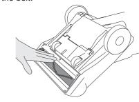
6 Refit the brush guard with 6 retaining screws.
