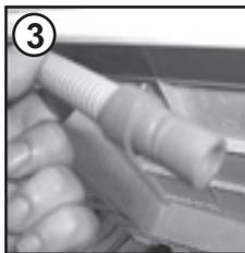
4. Attach the black hose from the kit, (using the connector and pipe clips supplied), to the hose removed from the bridge connection.
