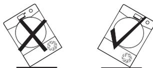
**CAUTION:** If the product is in different side, wait at least 4 hours before switching on so that the oil can flow back into the compressor. Failure to do this could result in damage to the compressor.
