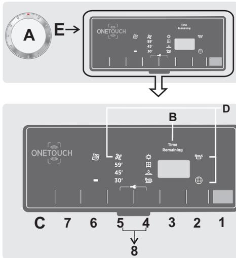
**A-Programme Selector** - Rotating the knob in both directions it's possible to select the desired drying program. To cancel the selections or switch off the dryer rotate the knob on OFF.
