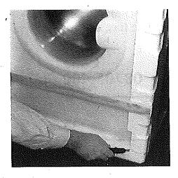
Remove the machine from its packaging close to the final location of the machine.
