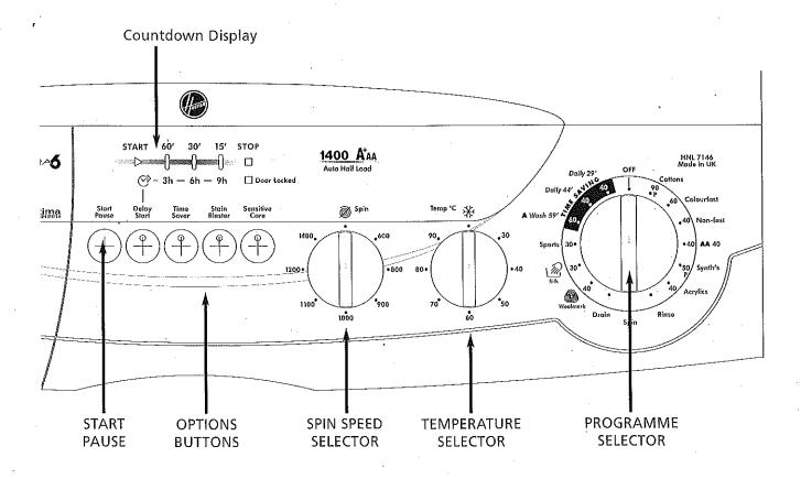
The programme selector must be return to the OFF position to reset the controls between each wash cycle.
