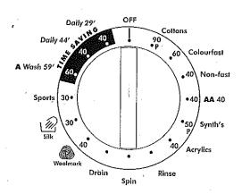
For handling the various types of fabric and their level of soiling in your laundry the washing machine has different programme groups according to type of wash, temperature, spin speeds and duration (see Programme Guide).
