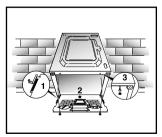
**Step 4**. Tilt the machine forward and apply the insulation base panel (corrugated plastic) to the base of the machine using the self-adhesive strips.
