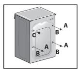
**Step 3**. Remove the 3 retaining screws (A) at the rear of the machine, as indicated in the image on the left.
