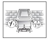
**Step 4**. Tilt the machine forward and apply the insulation base panel (corrugated plastic) to the base of the machine using the self-adhesive strips.
