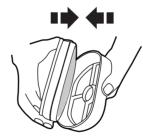
**IMPORTANT!** For optimum performance, shake off excess dust from the filters regularly. We recommend that the flexible HEPA filter pad is washed every 3 MONTHS.
