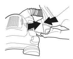
Insert the internal power plug on the main body into the YELLOW socket located in the neck of the cleaner.
