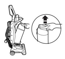
Hold the container using the carry handle over the bin and press the bin empty button. The dust container door will automatically open.
