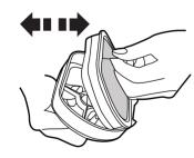
Wash the flexible HEPA filter pad thoroughly under hand warm water, gently squeezing the pad until the water runs clean.
