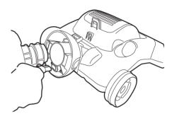
Attach the connector hose to the foot of the cleaner.
