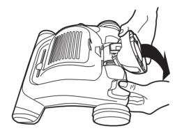
Ensure both halves of the neck are pushed together and the locking clips are fully engaged.
