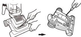
Hold the brush assembly and stretch the belt until the brush can be slotted back into the cleaner housing.
