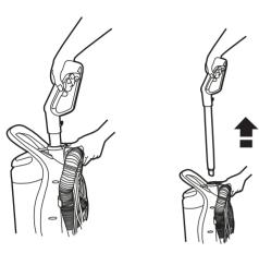
Remove the hose from the foot of the cleaner and insert into the removable handle / Crevice tool.
