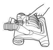
Wash the exhaust filter under hand warm water until the water runs clean. Remove excess water by shaking and leave to dry for 24 hours. Refit filter only when completely dry. DO NOT USE HOT WATER OR DETERGENTS.
