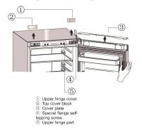
Note: Please hold the refrigerator door by hand during step 2 to prevent door dropping.
