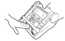
Remove brush assembly and check for wear on the belt. Loop the new belt around the motor and brush assembly.
