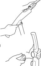
Check the hose by removing it from the cleaner, stretching it to full length.
