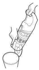
Once emptied, gently tap or shake the container to release any excess dust.
