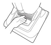
Remove the exhaust filter.
