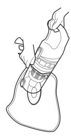
Press the bin empty button to empty the dust into the plastic bag. Close the bag quickly and dispose of it immediately.
