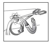
**Step 2**. Carefully cut through the hose-retaining clip at the rear of the machine, taking care not to cut the hose itself.
