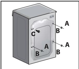
**Step 3.** Remove the 3 retaining screws (A) at the rear of the machine, as indicated in the image on the left.
