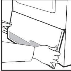
2. Turn the two locking levers anti-clockwise and pull out the condenser.
