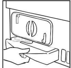
3. Open the lid located on the top of the container and empty the water.
