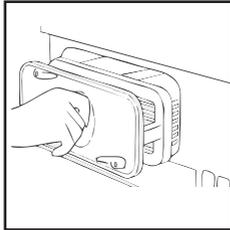
5. Refit the condenser ensuring it is in the correct way (as indicated by the arrow) and pushed firmly into place. Lock the two levers by turning them clockwise.
