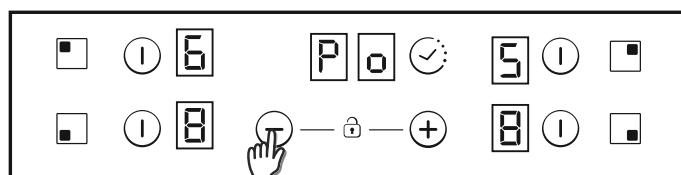
5.- Using 'Plus' and 'Minus' keys Power management value can be adjusted. In this example case between 6500 and 2500w. When required value is selected, touch at the same time 'Plus' & 'Minus' keys during 5 seconds.
