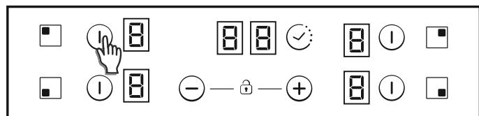
To switch ON a heater Touch any heater's zone during 400 msec. Long beep will be heard and "0" value will appear in target zone digit, indicating power level.
