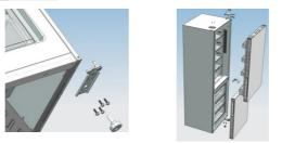
c. Remove the adjustable front feet under the lower hinge; use a tool to remove the 4 screws from the lower hinge and then disassemble the lower hinge. Door disassembly is finished.
