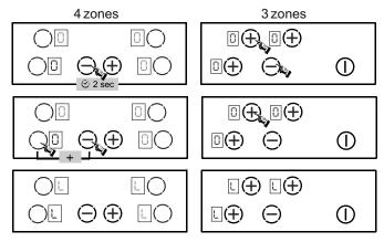
. The hob is locked, the locking indicator " L " is displayed on all zones for 20 seconds.
