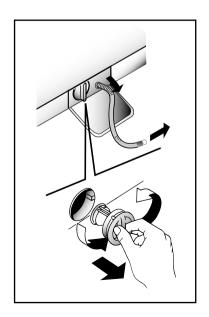
**Step 4**. Turn the filter anti-clockwise until it stops in the vertical position. Remove the filter and clean.
