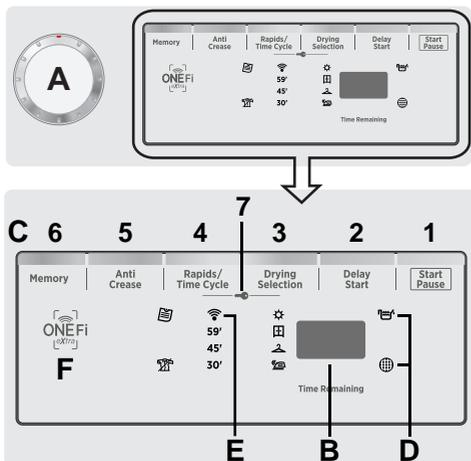
**A - Programme Selector** - Rotating the knob in both directions it's possible to select the desired drying program. To cancel the selections or switch off the dryer rotate the knob on OFF.
