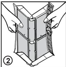
4. Snap the filter together and push back into place.
