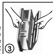
4. Remove the sponge gently from its place and then wash the sponge by holding it under a running tap turning it so to remove any dust or fluff.
