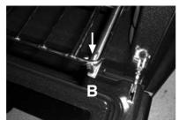
SLIDE OUT THE RUNNERS AND POSIZION THE SHELF SUPPORT **B** BEHIND THE SHELF SUPPORT B BEHIND THE SHELF STOP LOCATED AT THE FRONT SIDE OF THE KIT.
