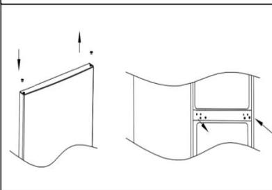
6. Install the bottom hinge to the left side of cabinet, then install two adjustable feet on the current position, then install the freezer door.
