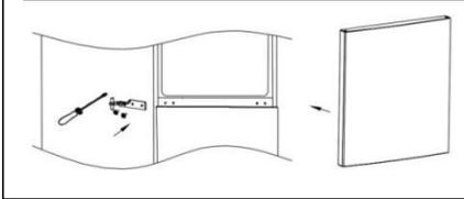
8. Remove the left hinge hole cover to right side, then install the upper hinge and hinge cover on the left side of cabinet.
