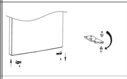
5. Remove the hinge hole cover from right side of freezer door, then install to left side. Remove the center hinge screw cover on the left side of cabinet, then install its to right side of cabinet.
