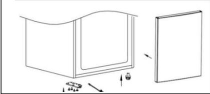
7. Install the center hinge to the left side, then install the fridge door at the same time.
