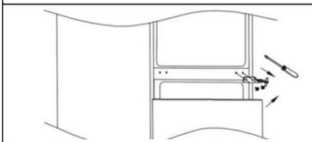
3. Remove the screws that secure the lower hinge to the right side of the cabinet, then the hinge and adjustable feet.
