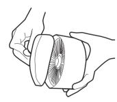
Wash the GREY foam filter thoroughly under hand warm water until the water runs clean.
