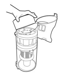
Separate the GREY foam filter from the BLUE HEPA filter pack using the tab provided. Gently tap both filters against the side of a bin to release excess dust.
