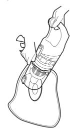
Press the bin empty button to empty the dust into the plastic bag. Close the bag quickly and dispose of it immediately.
