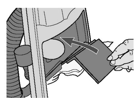
Push the bag collar over the hose inlet until it is firmly in place.
