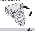
Open clip and lift cover to remove blockage.
