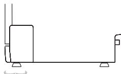
Once the appliance is positioned, adjust the feet (screwing them in or out) to adjust the height of the dishwasher, making it level. In any case, the appliance should not be inclined more than 2°.
