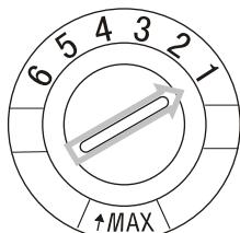
A measured amount of rinse aid is released during the final rinse. As with detergent, the amount of rinse aid needed for your dishes depends on the hardness of the water in your area. Too much rinse aid can result in lather or foaming and cause cloudiness or streaks on your dishes. If the water in your area is very soft, you may not need rinse aid. If you do, you can dilute the rinse aid with an equal amount of water.
