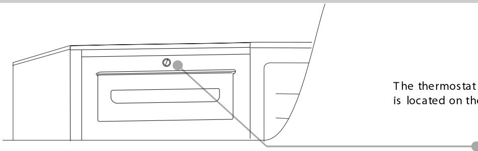
The thermostat unit to control the appliance is located on the right of the top cover.
