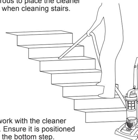
ALWAYS work with the cleaner below you. Ensure it is positioned up against the bottom step.
