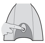
Push bottom of the On/Off switch to switch on. Push top of the On/Off switch to switch off.
